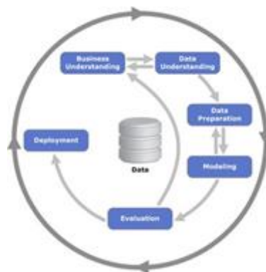
Gambar 1. CRISP-DM ( Cross-Industry Standard Process for Data Mining )
